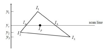
$$\begin{split} I_{a} &= I_{1} \frac{y_{s} - y_{2}}{y_{1} - y_{2}} + I_{2} \frac{y_{1} - y_{s}}{y_{1} - y_{2}} \\ I_{b} &= I_{1} \frac{y_{s} - y_{3}}{y_{1} - y_{3}} + I_{3} \frac{y_{1} - y_{s}}{y_{1} - y_{3}} \\ I_{p} &= I_{a} \frac{x_{b} - x_{p}}{x_{b} - x_{a}} + I_{b} \frac{x_{p} - x_{a}}{x_{b} - x_{a}} \end{split}$$
