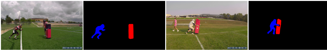
Fig. 4: Examples of mask segmentation results. The first and third images from the left represent the original images while the other two images are the output of the mask segmentation of the corresponding images.
