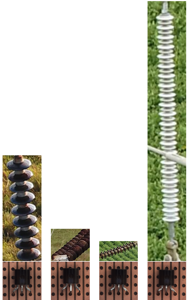
Figure 4: Undamaged insulators (top) and transistors (bottom)
